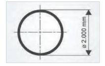
CPCut's cantilever design with open loading area and a powerful chuck enables clamping and processing of pipes and profiles up to Ø 2,000 mm.
