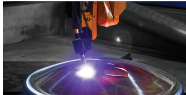
Tank end processing on DRM, with a 3D rotator with tilt angle up to 120°
