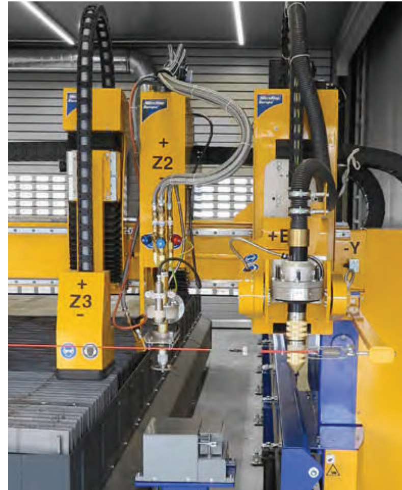
Configuration of MasterCut machine with a bevel head, an oxyfuel torch and a punch marker
