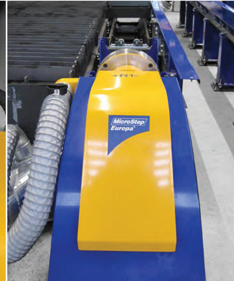
This pipe cutting device can process pipes up to Ø 300 mm
