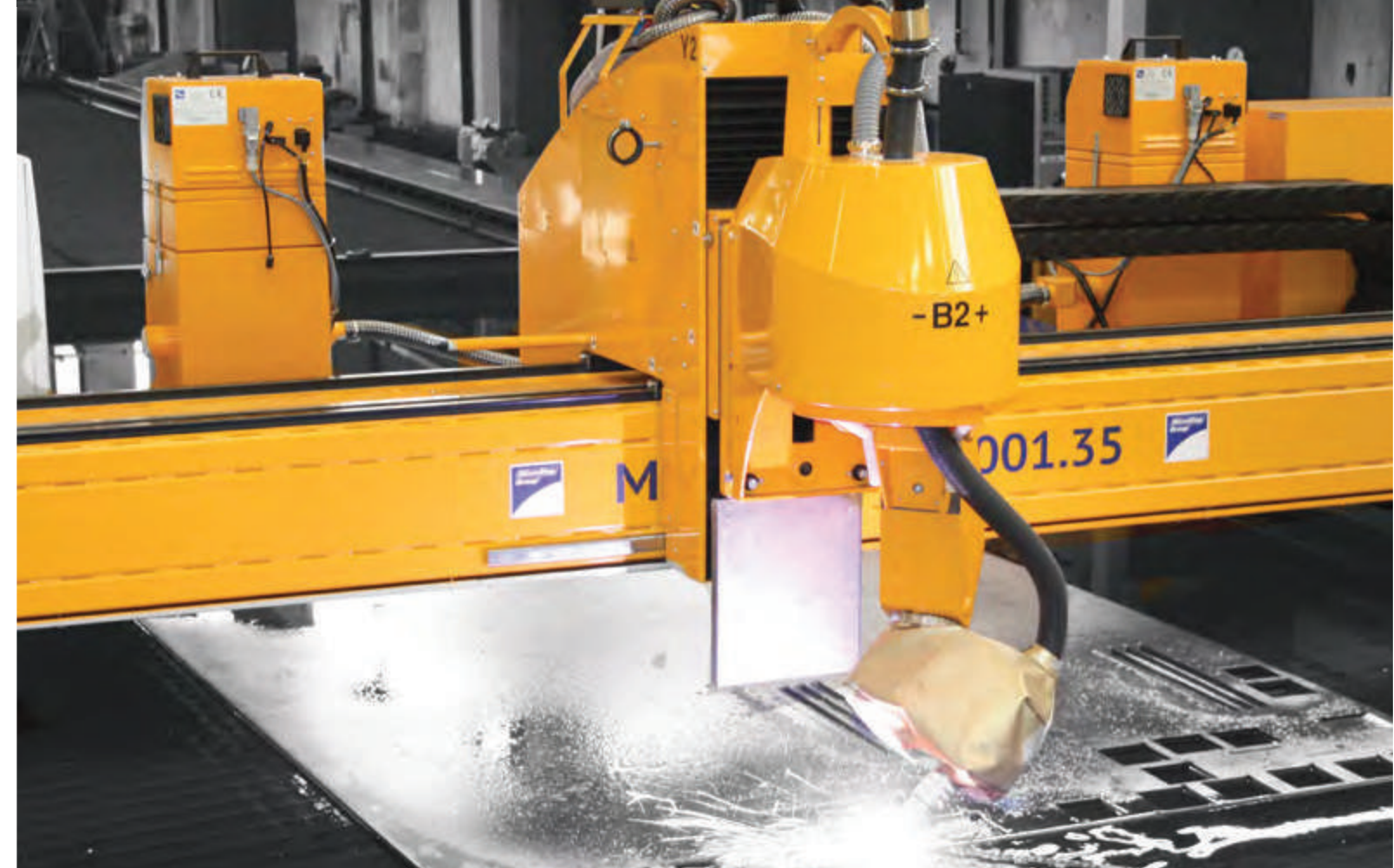
Plasma rotator performing bevel cutting on a water table
