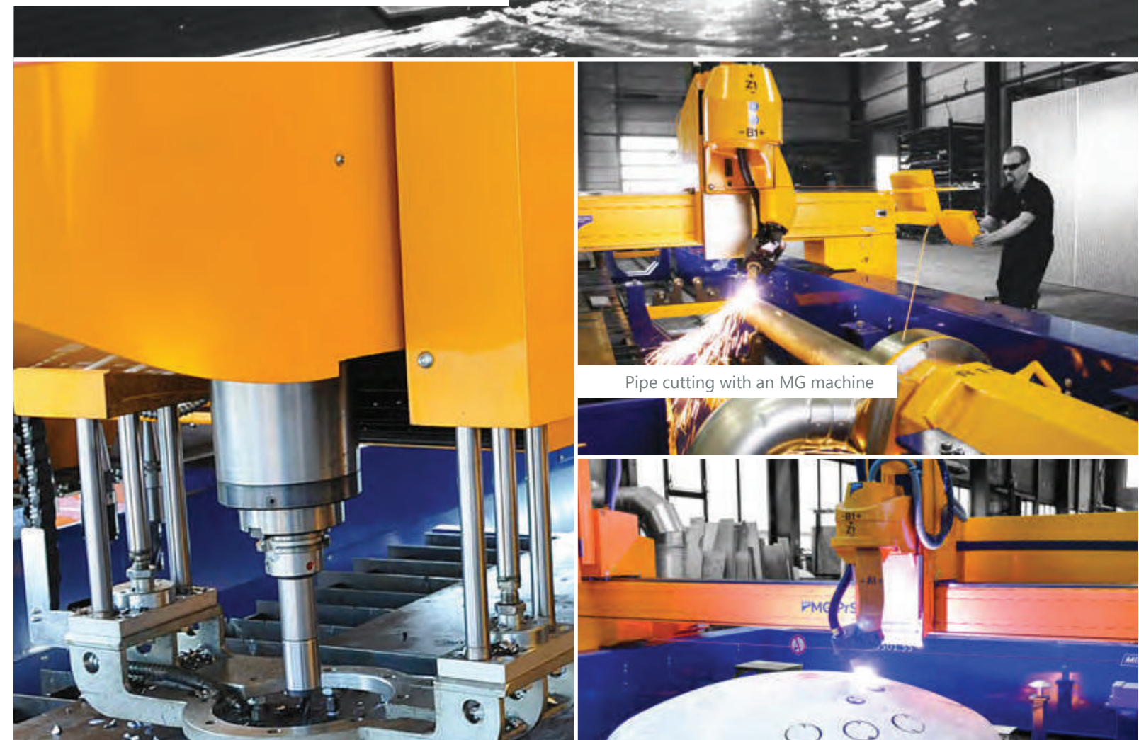
The powerful drilling head enables drilling, tapping, and countersinking
